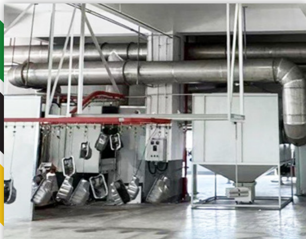
Powder coating is used to prevent corrosion of the steel during operating lifetime.
